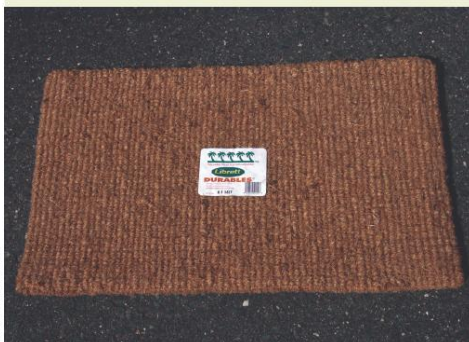
Figure 4-7 Coir fibers are often used in things like floor mats because they are so durable.
